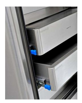
• Telescopic slides simplify the process of putting modules in and out of the chassis.
