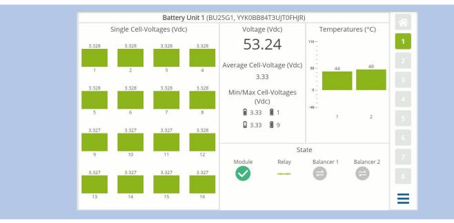
A battery module contains two battery blocks with each eight cells. The more detailed view into the single Battery Modules allows a closer look at each cell, its voltage and the temperature of each Battery block.
